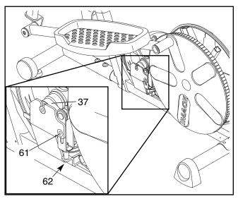
Next, loosen the M8 x 19mm Flat Head Bolt (61) and turn the Adjustment Screw (62) until the Belt (37) is tight. Once the Belt is tight, tighten the Flat Head Bolt. Then, reattach the side shields. Note: If you have questions regarding which screw should be in which hole, see EXPLODED DRAWING B on page 19 and the PART LIST on page 17.
